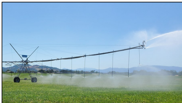
New gravity pressurized, efficient, center pivot sprinkler system
